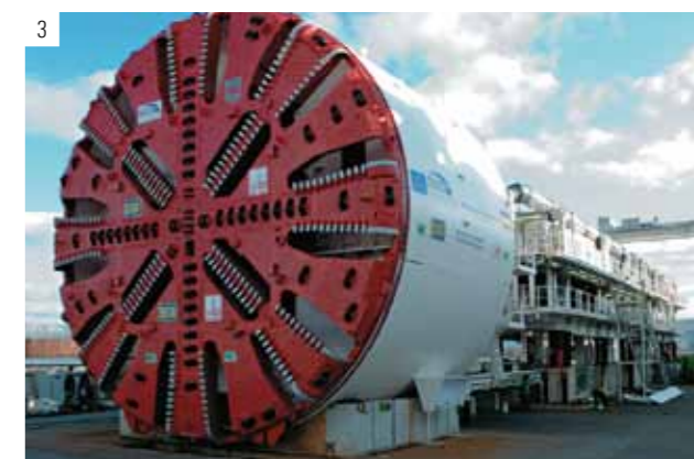
1 Gdansk inner port shipyard looking downstream to the future tunnel crossing 2 Port at the area of the link 3 TBM mix-shield 13 m diameters – comparable type of the company Herrenknecht
